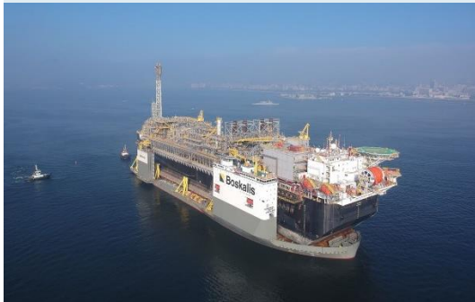
MWS for transportation of FPSO P-67 from China to Brasil
